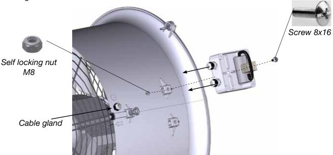
4. Bring the motor cable through the cable gland and make the electrical connection to the terminal block as follows:
