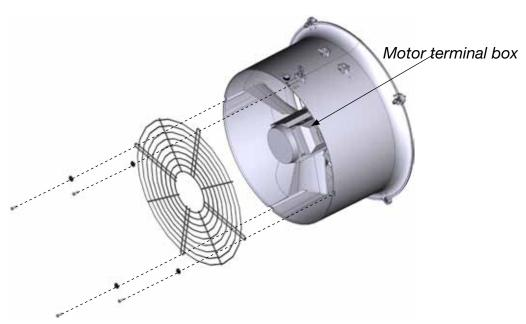
2. Open the motor terminal box cover and change the position of the connection plates from Star to Delta. Tighten the connection nuts with a torque of 3 Nm (tight but not too much) and close the cover:
